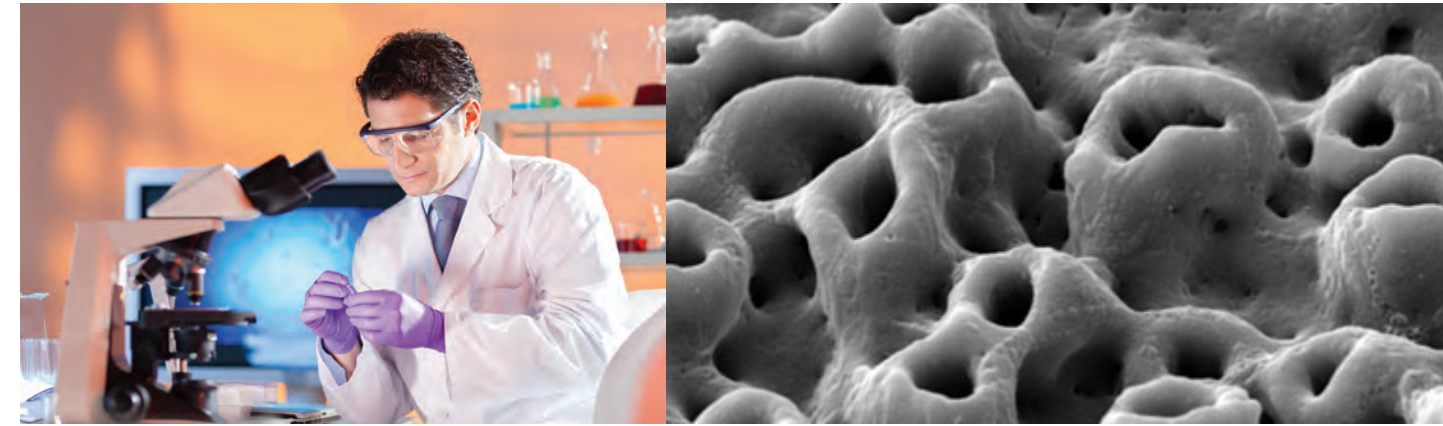
Implant after machining and washing is reasonably clean and mostly free from foreign particles, enabling good conditions for further stages of the surface treatment.
